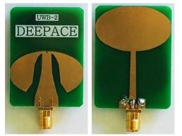
The two images at the left are of the front and back sides of this PCB antenna. The right-hand image needs to be imagined as having been printed exactly behind the lefthand image.
