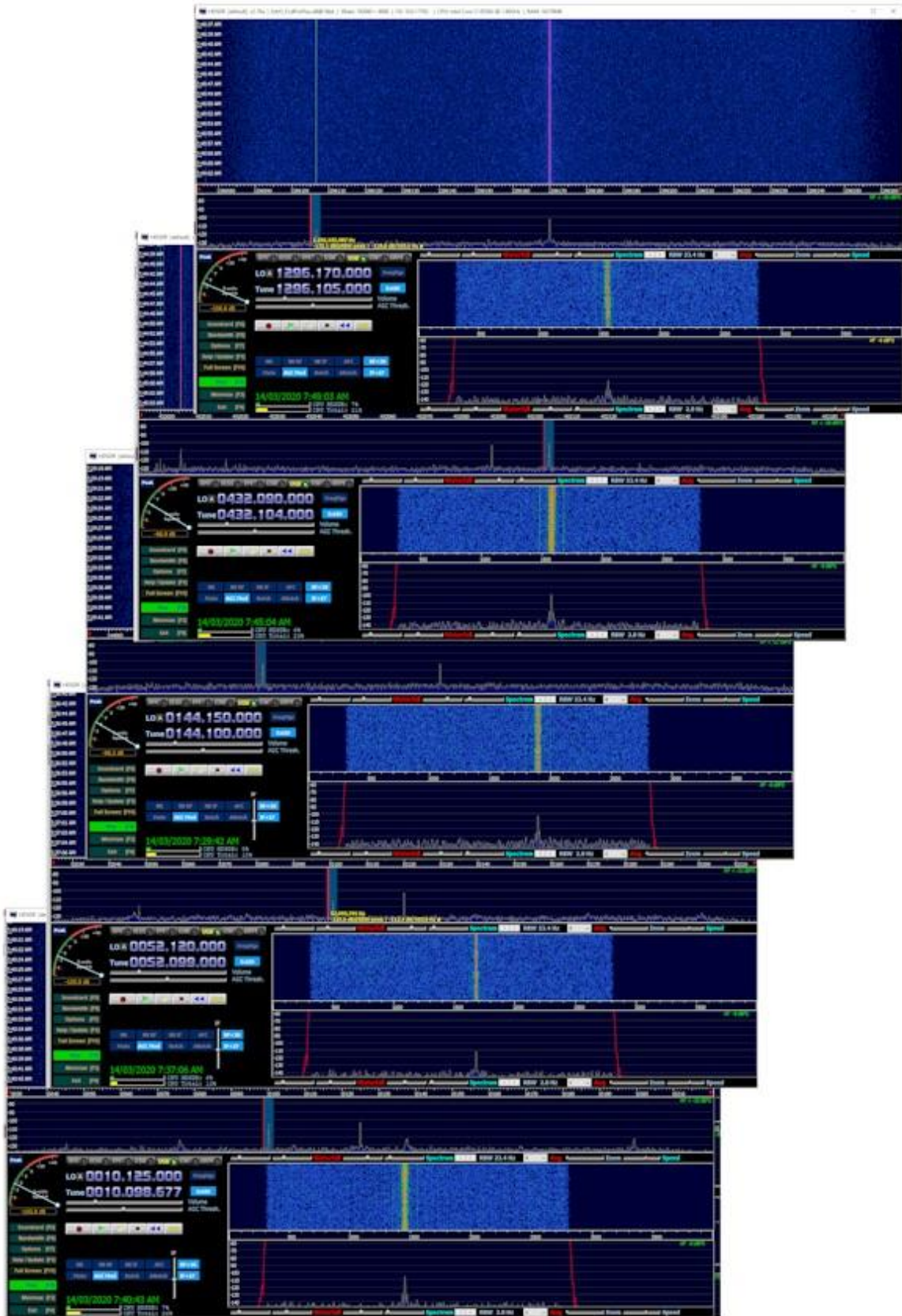
Figure 7 Screen dumps HSDR IC9100 bands HF through 1296 MHz
