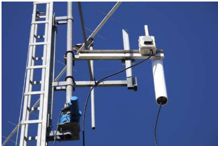
Closeup photo is the 24GHz PA and slot antenna.
