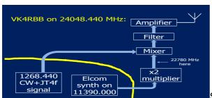
Similarly, as per the 10 GHz stage, the 1268.440 is mixed with the doubled output of the Elcom synth to produce 24048.440 MHz.
