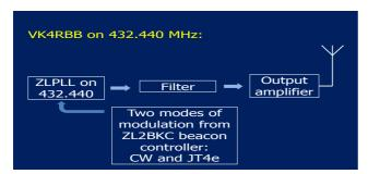
The simplest block is a direct output from a ZL-PLL into an amplified via a low pass filter.
