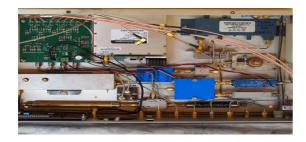
The photos above show the main box containing the 10 MHz distribution, Elcom synthesiser and all of the ground level mixing stages. The LCD is connected to the ZL2BKC beacon controller.
