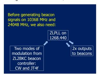
A separate ZLPLL generates 1268.440 for use by the 10 and 24 GHz stages
