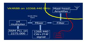
The 10 GHz masthead amplifier power is feed into the low loss coaxial feed.
