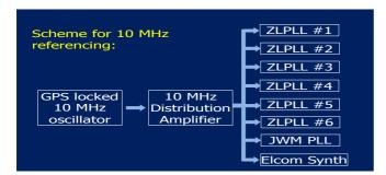
Eight signal sources in total frequency disciplined by a single 10 MHz source distributed amplifier.
