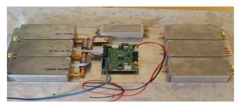
Separate 2RU boxes contain the ground level located power amplifier stages.
